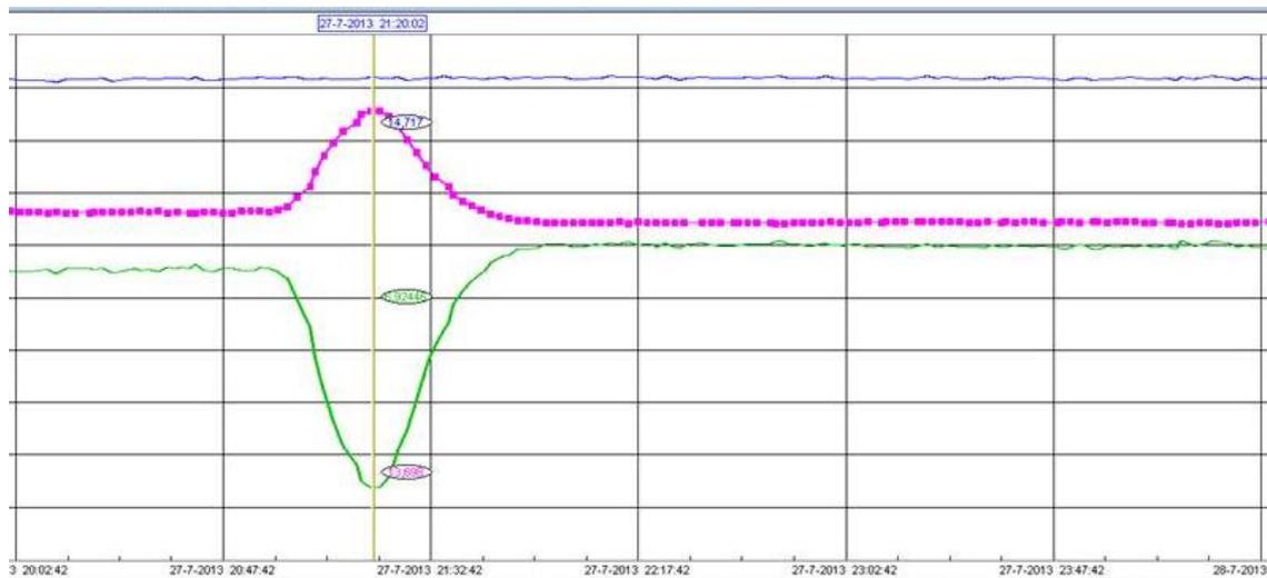
**Figure 6-19** Screenshot from Waternet SCADA Interface, Showing a Failure in Ozone Supply (green) and Coinciding Increase in the UV Parameter (blue) Indicating the Change in Absorption due to Ozonation Decrease.  $\Delta UV$  is Related to the Amount of Organic Material that has Reacted with Ozone, and therefore an Indicator of the Amount of Ozone Dosed. The Failure Was Detected Based on  $\Delta UV$  Before the Control Room Reported the Issue.
